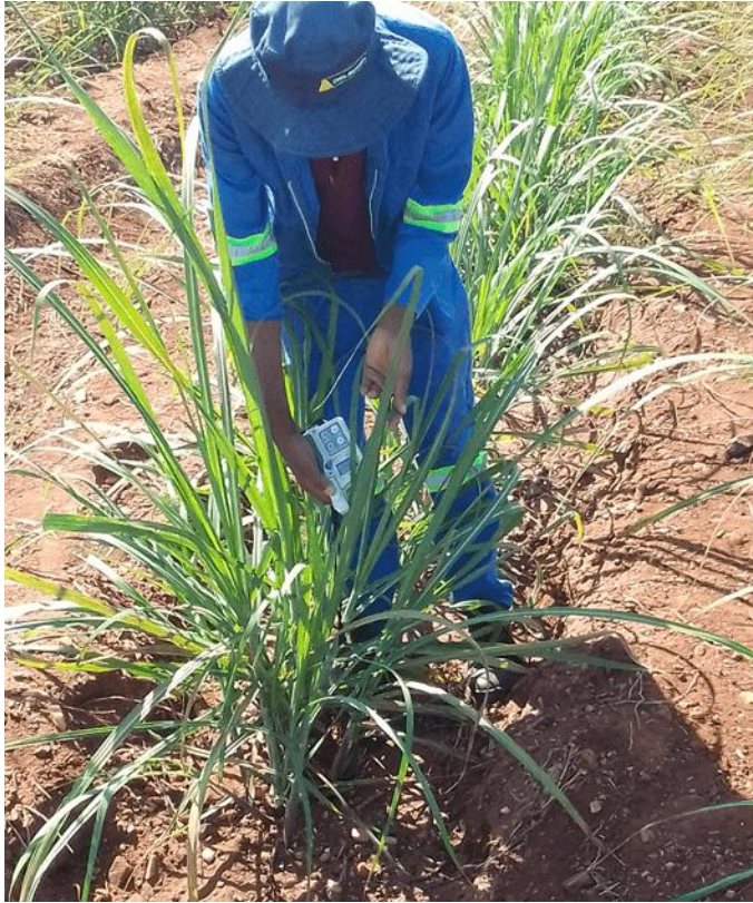
Figure 5.2: Chlorophyll content determination with a SPAD meter on sugarcane crop. Source (This study)
