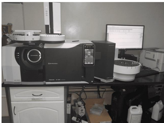
Figure 6.3: Shimadzu Nexis GC2030, GCMS TQ8040NX Triple Quadrupole Mass Spectrometer, HS-20NX mode. Source (This study)
