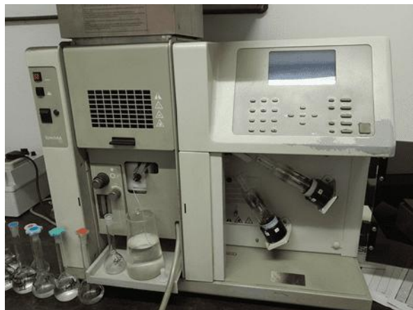
Figure 4.5: Atomic Absorption Spectrometer used in measuring potassium, calcium, and magnesium. Source (This study)
